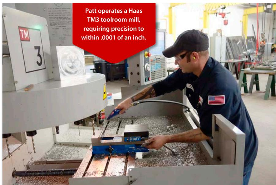
Patt operates a Haas TM3 toolroom mill, requiring precision to within .0001 of an inch.
